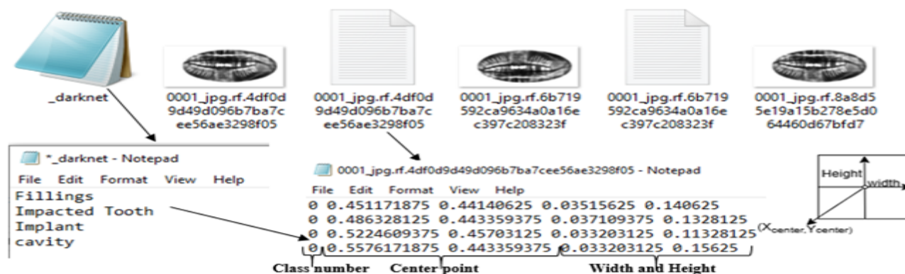
Figure 3: Image and bounding box dimensions in TensorFlow format.
