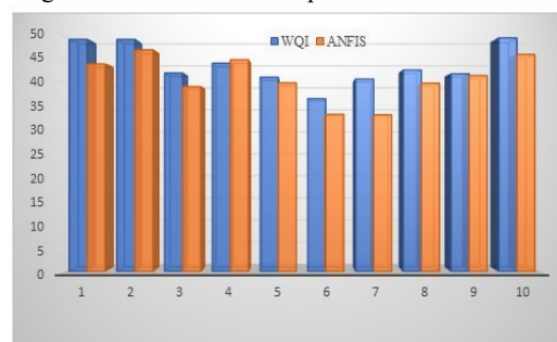
Figure 4: Comparison between measured WQI (blue bars) and predicted WQI using the ANFIS-D model (orange bars) across 10 sampling points.
